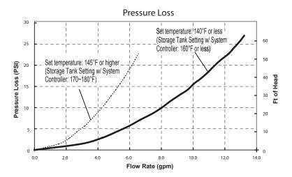
**NOTE:** For Quick-Connect and Multi-System installations, pressure loss remains constant throughout the system regardless of the number of units installed. Multiply the total number of units in the system by the required flow rate from each unit to determine the total pressure loss from the chart above.
